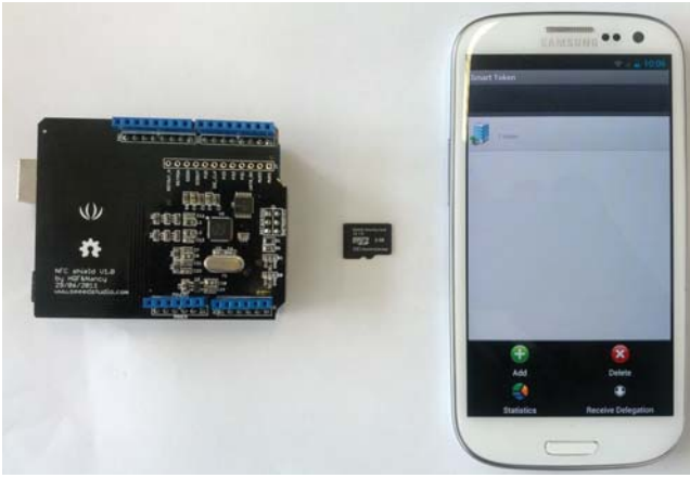
Figure 4: Prototype setup consisting of an Arduino Uno board with NFC shield, a secure microSD smart card and a Samsung Galaxy S3 smartphone (left to right).
